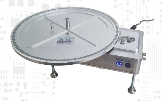
Our ZB-REV2.0 autosampler features an extreme sealing surface (70 mm) and a separate purging chamber. Thus, samples are already transferred into this purging chamber before the measurement and continuously purged with helium over the period of the preceding measurement. Due to the large sealing surface of the rotary turret (approx. 70 mm) and these additional purging, a **ZERO blank measurement** can be ensured without restricting the operating comfort.
